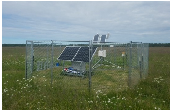
A meteorological station for the Midnight Solar project collecting solar performance data.
