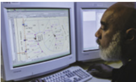
Geographic Information System software allows computer access to layers of data on Chugach's primary distribution system. Technicians can easily update, analyze, map, and integrate information such as Chugach's customer information or municipal assessor data.
